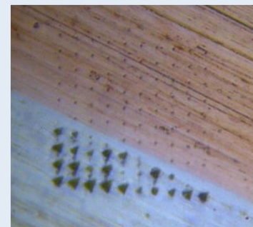
Figure 7 shows a grid of indents taken across a Sn/Cu solder joint at elevated temperature.
