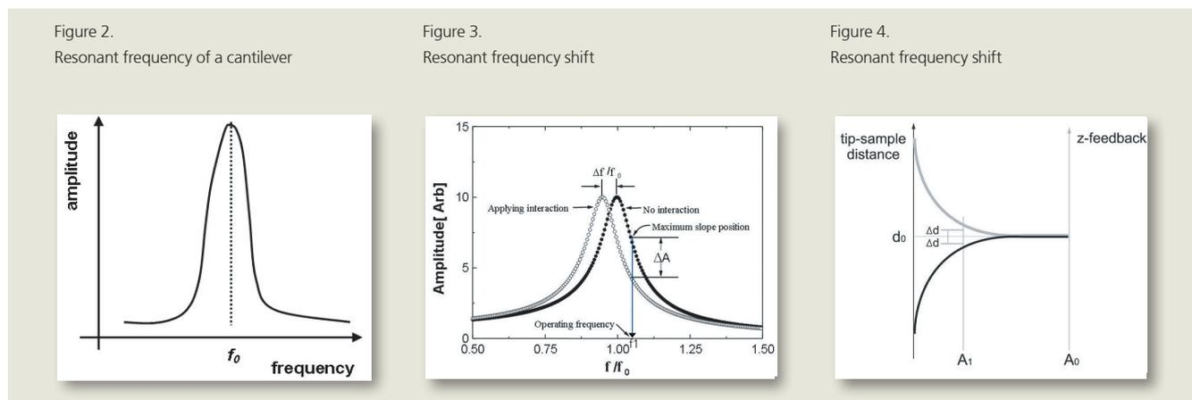
On the other hand, the spring constant affects the resonant frequency ( $f_0$ ) of the cantilever, and the relation between the spring constant ( $k_0$ ) and the resonant frequency ( $f_0$ ) in free space is shown as in Equation (2).
