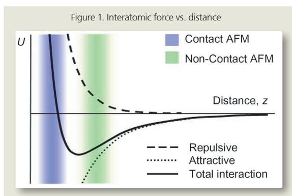
Because of the attractive force between the probe tip and the surface atoms, the cantilever vibration at its resonant frequency near the sample surface experiences a shift in spring constant from its intrinsic spring constant ( $k_0$ ). This is called the effective spring constant ( $k_{eff}$ ), and the following equation holds:
